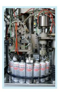
iBiotec is equipped with 3 fully automated filling lines with a combined capacity of 60 aerosol containers per minute per machine.
