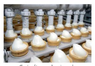
Cleaning of ice-cream dispensing nozzles ensures constant dispensing rate and weight.
