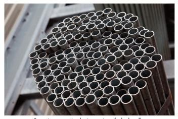
Corrosion protection by immersion of tube bundles.
