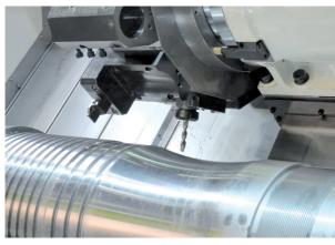
Pilot hole drilling with classic drill chuck and bits on both concave and convexed surfaces.
