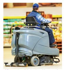
Cleaning of floors wih walk behind scrubbers or rider scrubbers, equipped with water flow control.
