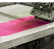
Washing of silk screens, cleaning of silicon elastomer pad printing stamps.
